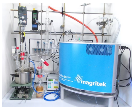
Fig. 1: Laboratory set-up for the monitoring of the dissolution kinetics of additives in trialkoxy silanes.
