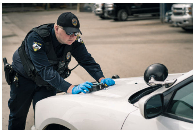
Figure 1. The right-angle attachment enables measurements to be conducted on surfaces.
