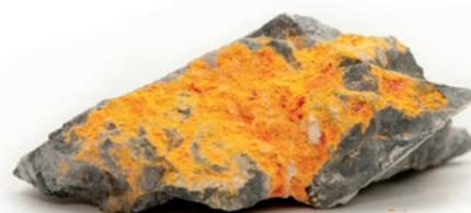
**Figure 1.** Arsenic is not usually to be found in its pure form in nature. One of the compounds frequently encountered is realgar ( $\text{As}_4\text{S}_4$ ), here seen on a substrate of stibnite and granite.
