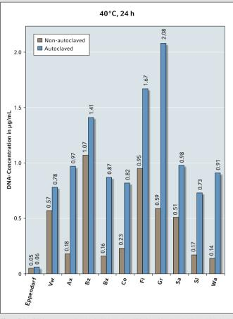
Fig.1: False DNA concentration ( $\mu$ g/mL) based on UV-absorbing leachables, which had been released from micro test tubes into ultra-pure water samples after incubation at 40°C, 24 h. Mean values of 24 pooled samples from non-autoclaved (brown bars) and autoclaved (blue bars) tubes are shown.
