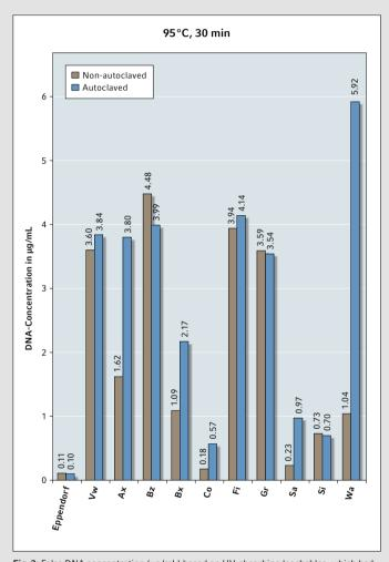
Fig. 2: False DNA concentration ( $\mu$ g/mL) based on UV-absorbing leachables, which had been released from micro test tubes into ultra-pure water samples after incubation at 95°C, 30 min. Mean values of 24 pooled samples from non-autoclaved (brown bars) and autoclaved (blue bars) tubes are shown.
