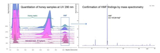
Figure 1: Fast and reliable HPTLC analysis of hydroxymethylfurfural (HMF) in honey samples
